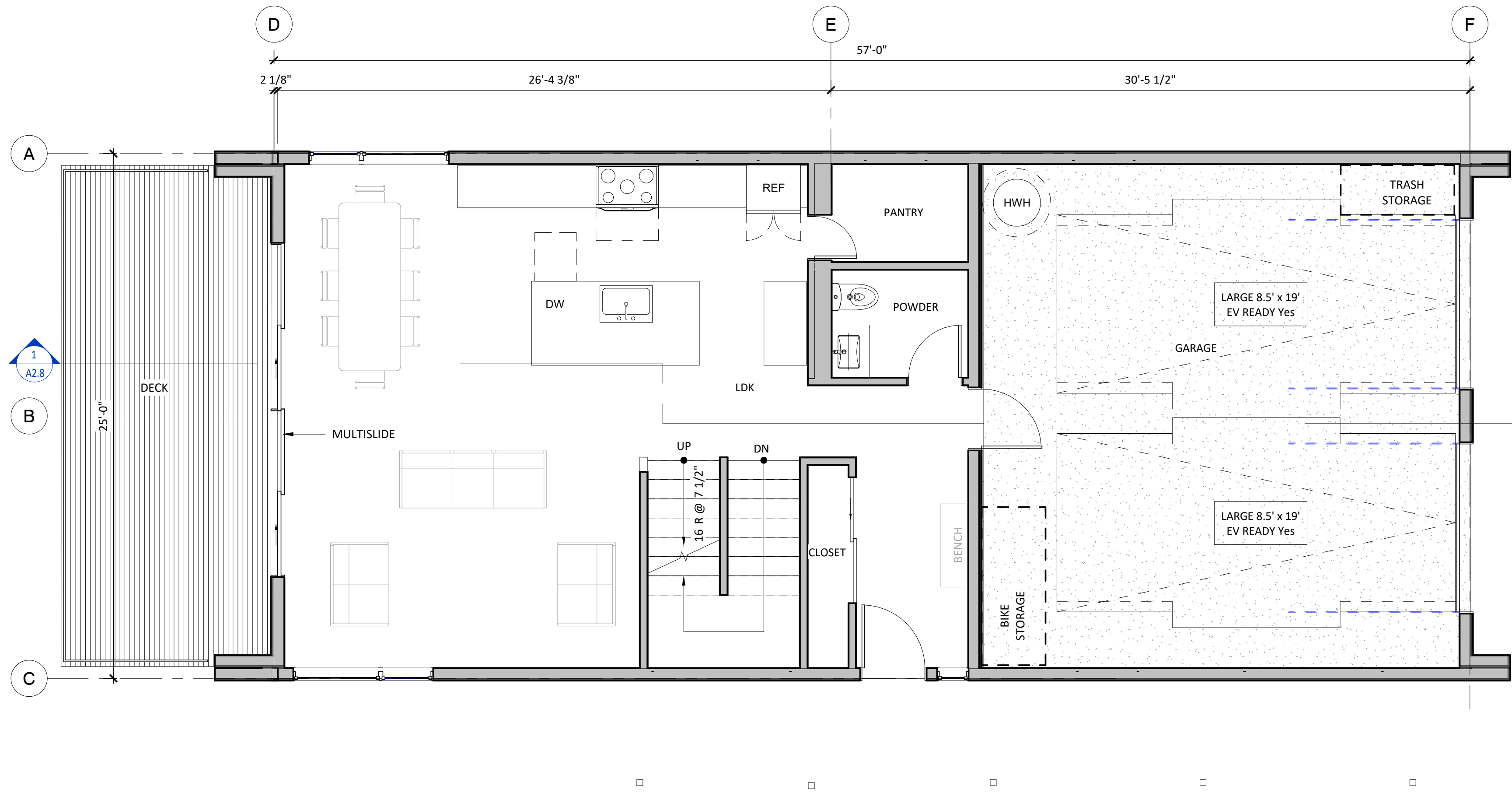
2 LEVEL 1 FLOOR PLAN - TYPE 2 1/4" = 1'-0"
