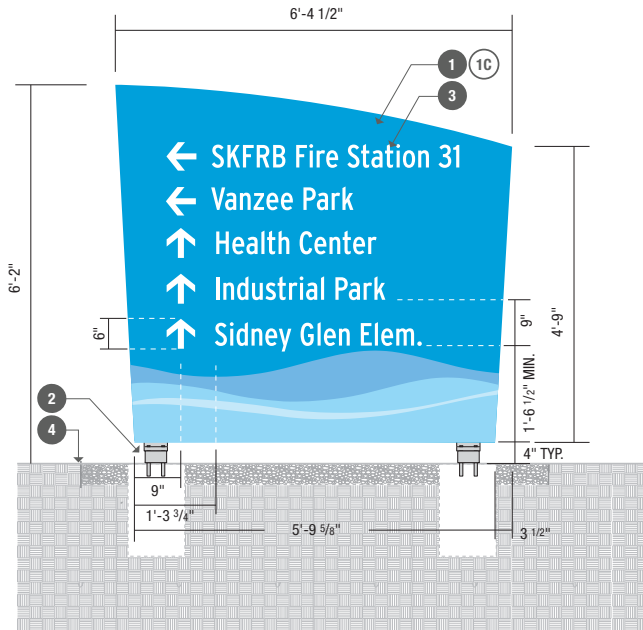
1 ELEVATION - Vehicular Trailblazer Sign / Primary 1/2" = 1'-0"
