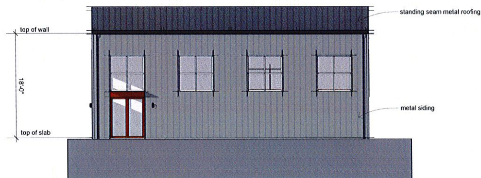
3 Side Elevations - Typical Shop Building 1/8" = 1' - 0"
