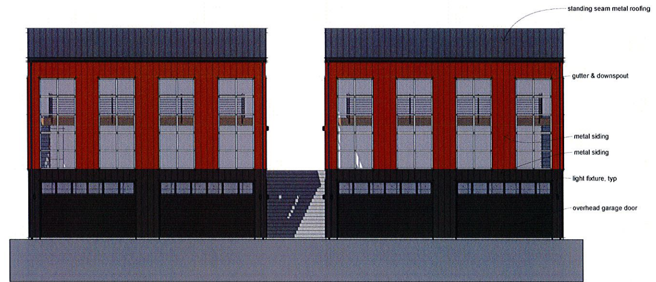
1 South Elevation - Buildings 1 & 2 1/8" = 1' - 0"
