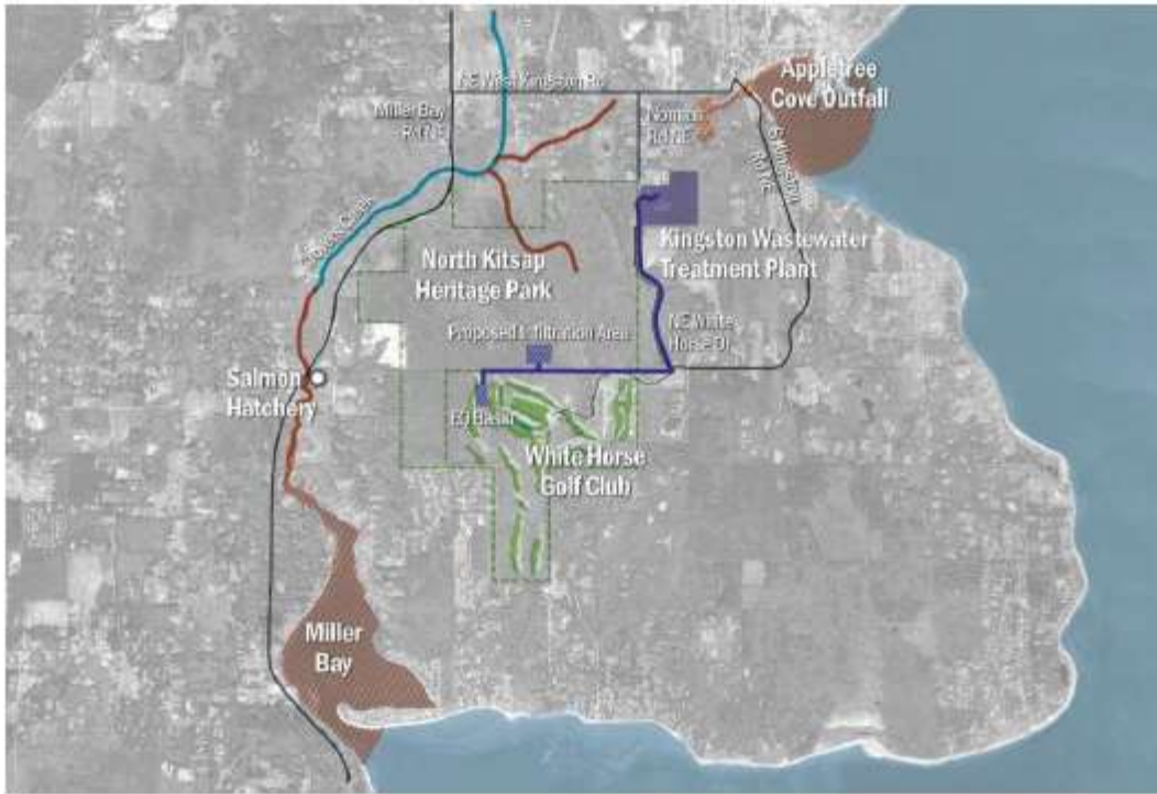
Figure 1. Location of pipeline to WHGC and to infiltration area (from Brown & Caldwell, 2019)
