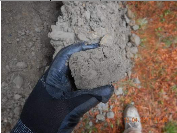
Photo TP-1A: View of fine SAND/silty SAND from about 9 feet below grade.
