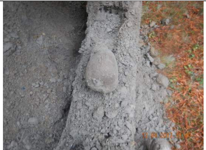
Photo TP-1B: Excavation spoils in backhoe bucket from 9 feet below grade.
