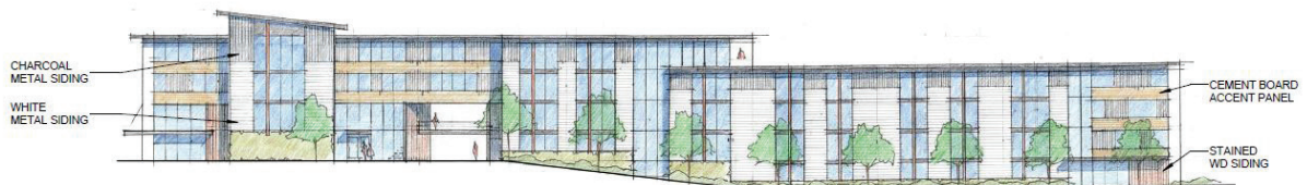
APARTMENT - NORTH ELEVATION
